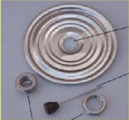
Lid with a hole drilled in its center
